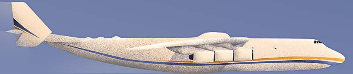
Antonov An-225 LENGTH: 84 m WINGSPAN: 88.4 m
