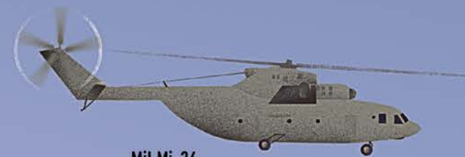
Mil Mi-26 LENGTH OF FUSELAGE: 33.7 m MAIN ROTOR DIAMETER: 32 m
