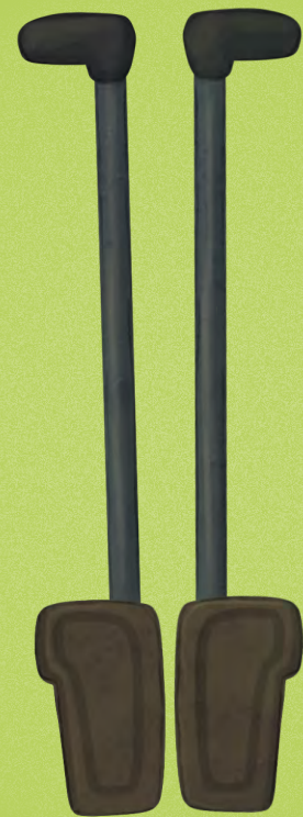
Left and right track travel levers. By pushing the levers apart you can make the caterpillar go straight ahead.
